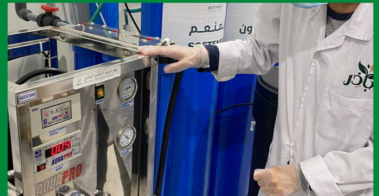
Reverse osmosis purification device in the Badir Smart Farm program, Badir Farm
